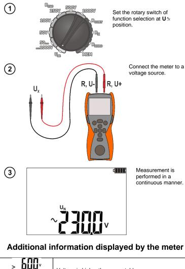
Voltage is higher than acceptable. Immediately disconnect the test leads.
