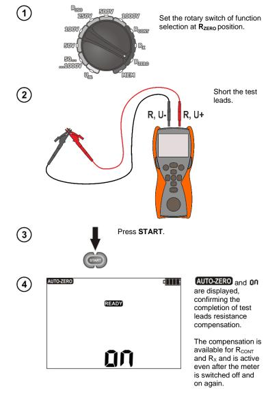
In order to remove the compensation made (and return to default calibration), perform the above-mentioned activities with test leads open – messages (AUTO-ZERO) and On disappear, the following message is displayed [JFF.]
