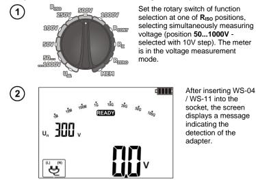
Set the measuring voltage  $U_N$  (applies only for 50...1000V position of the switch), and times t1, t2, t3 as in double-lead measurement. These settings relate to the measurement of insulation resistance for each pair of leads selected in the main settings.
