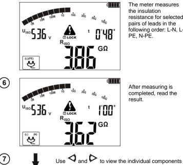
The meter measures the insulation resistance for selected pairs of leads in the following order: L-N, L-PE, N-PE.
